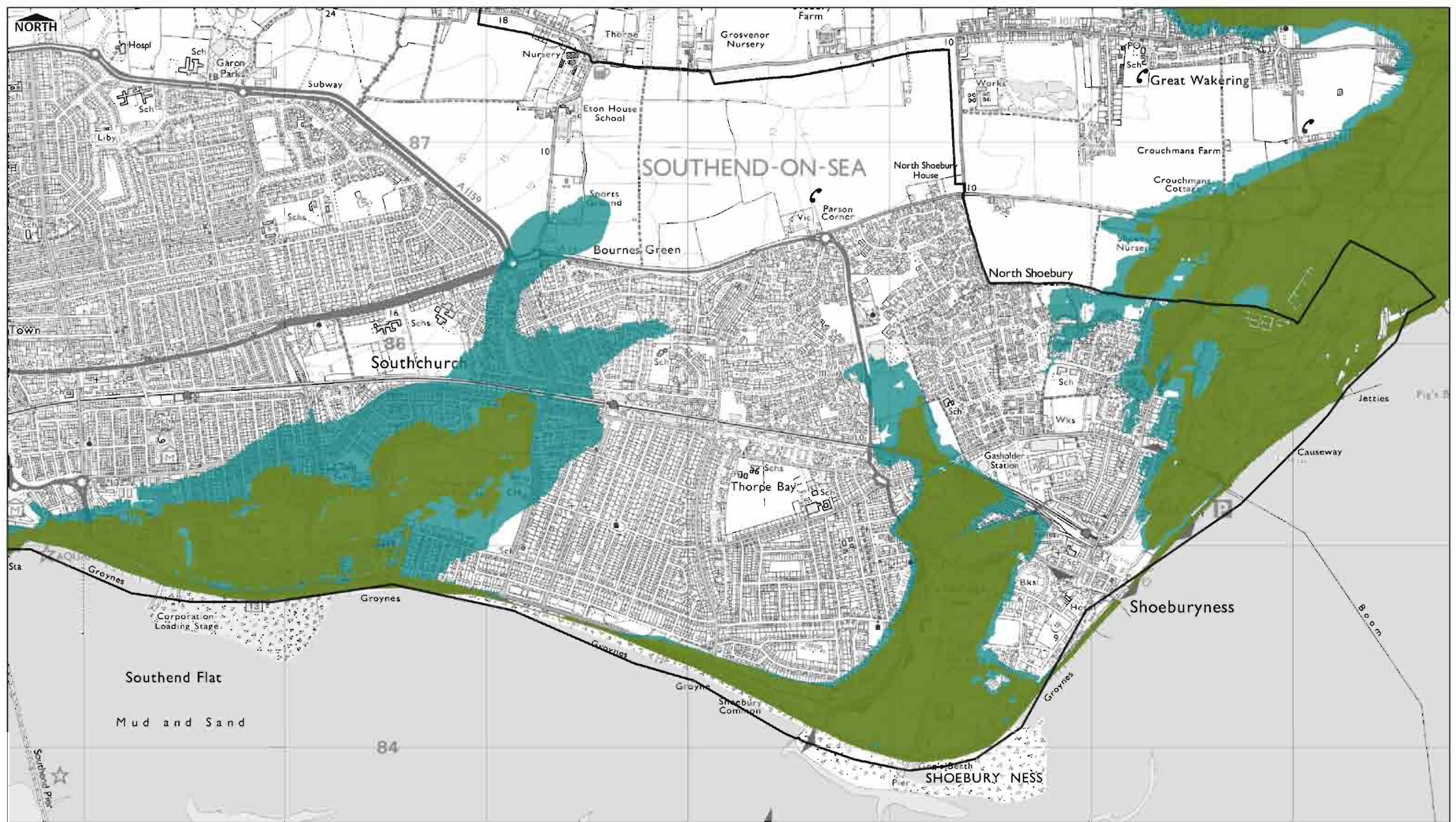
FIGURE 15 - MODELLED AREAS OF OVERTOPPING - EAST
